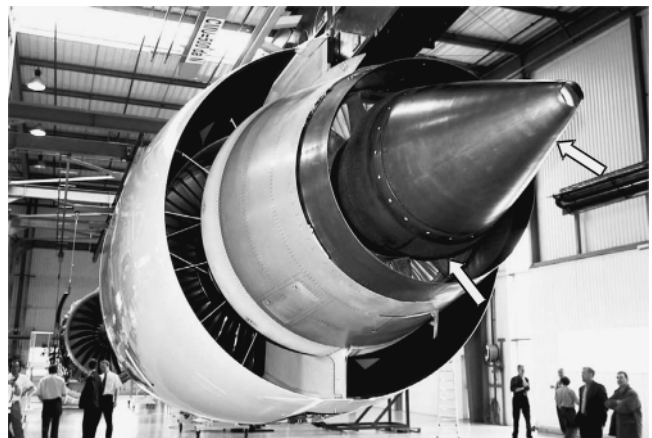
Fig. 8 TIMETAL 21S plug-and-nozzle assemblies (arrows) for the Trent 500 engine on the A340-500/600. The photograph is courtesy of Aeronca, Inc. (2000).
